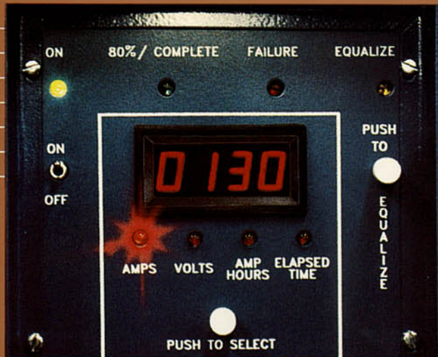
Output Amperes —displays actual output current within \pm 1 amp.
