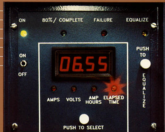
Elapsed Time —directly readable in hours and minutes.
