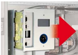
Control electronics are easy to remove.
